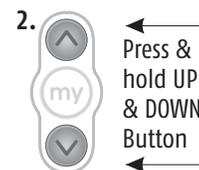
3) Press and hold either the **UP or DOWN button** on the transmitter to adjust shade to new position.
