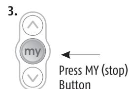
**Note:** Shade should be stationary prior to activating intermediate position function. If shade is actively moving (in-motion) MY (Stop) button should be pressed twice. To Delete: Activate shade to (IP) position, then press and hold the MY (Stop) button for 5 seconds.
